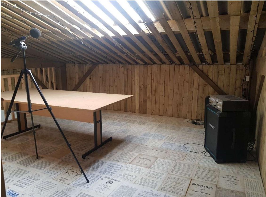
Picture 3: Source noise generated and repeated inside the barn on the 4<sup>th</sup> top landing.
