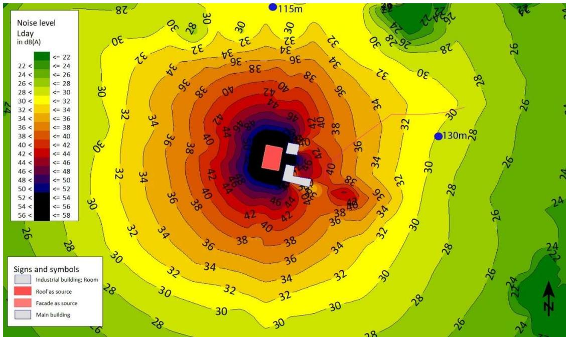
Noise map 2: This includes noise from inside the barn, noise around the pond equivalent to people speaking with a raised voice but not shouting. It also includes vehicles driving up the drive at a rate of 10min within the hour.
