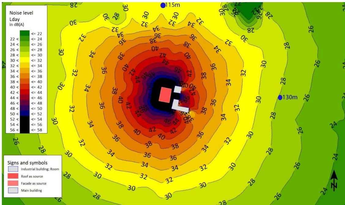
**Noise map 1:** Spread of noise from inside the barn at LAeq(1 hour 41Min) 79dB inside the barn. The blue circles are distance from the barn. The noise model includes the geometry and layout of the land. This does not include noise from celebrations around the pond or cars arriving.
