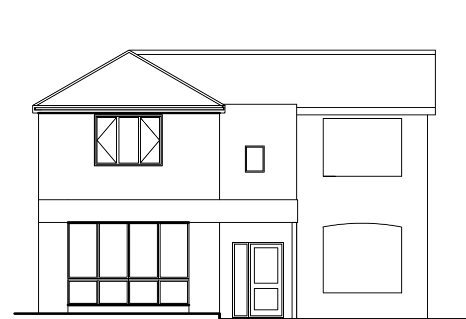
EXISTING FRONT ELEVATION
