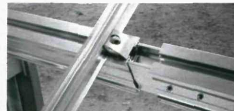
Carrier sections can be mounted even on connection points.
