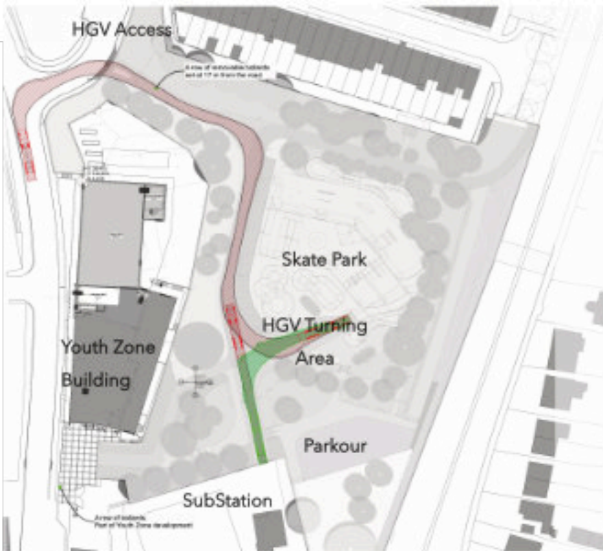
FIG 8. HGV Service Vehicle Swept Path
