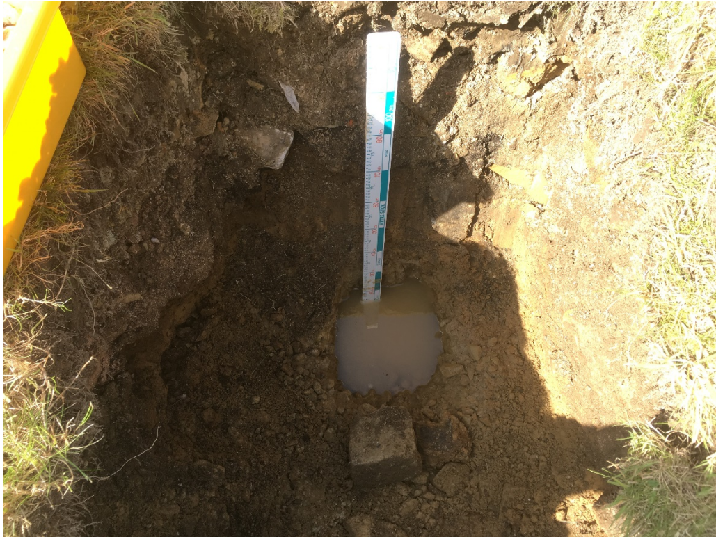
Photograph 7 – View of percolation testing being conducted in the base of FD101, from 0.8 to 1.1 m bgl. Facing approximately north.
