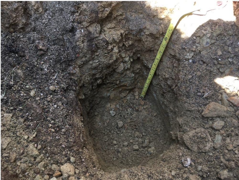
Photograph 6 – View of the 0.3 x 0.3 x 0.3 m hand pit excavated at the base of the FD101 trial pit, from 0.8 to 1.1 m bgl.
