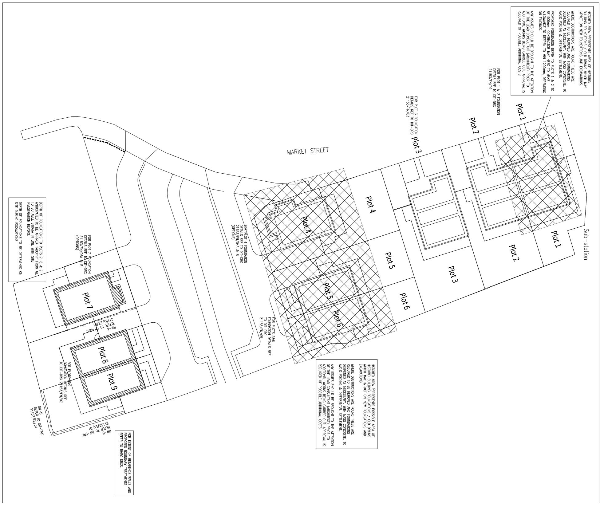
TYPICALLY ALL STRIP FOOTINGS TO BE SET CENTRAL ON WALL LINE, CHECK ARCHITECTS DETAILS FOR OVERALL WALL THICKNESS AND SETTING OUT
