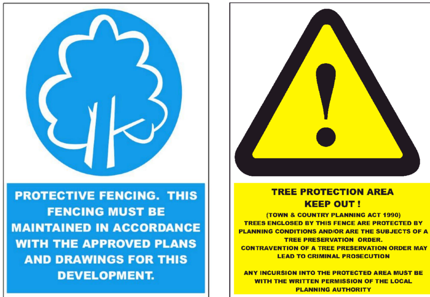
Figure 3: Example fence signage. Reproduced from BS5837:2005 © BSI.
