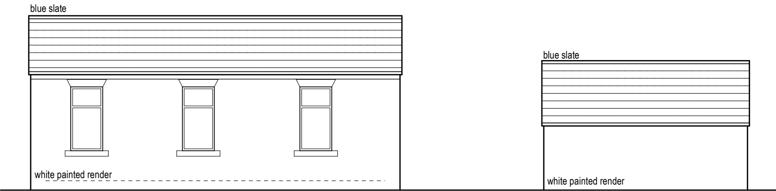
Existing rear elevation (1:100)
