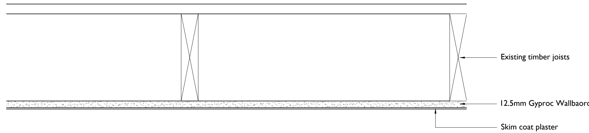
6 3200 CLG-10I Ceiling Detail as NBS K10/245 1:5
