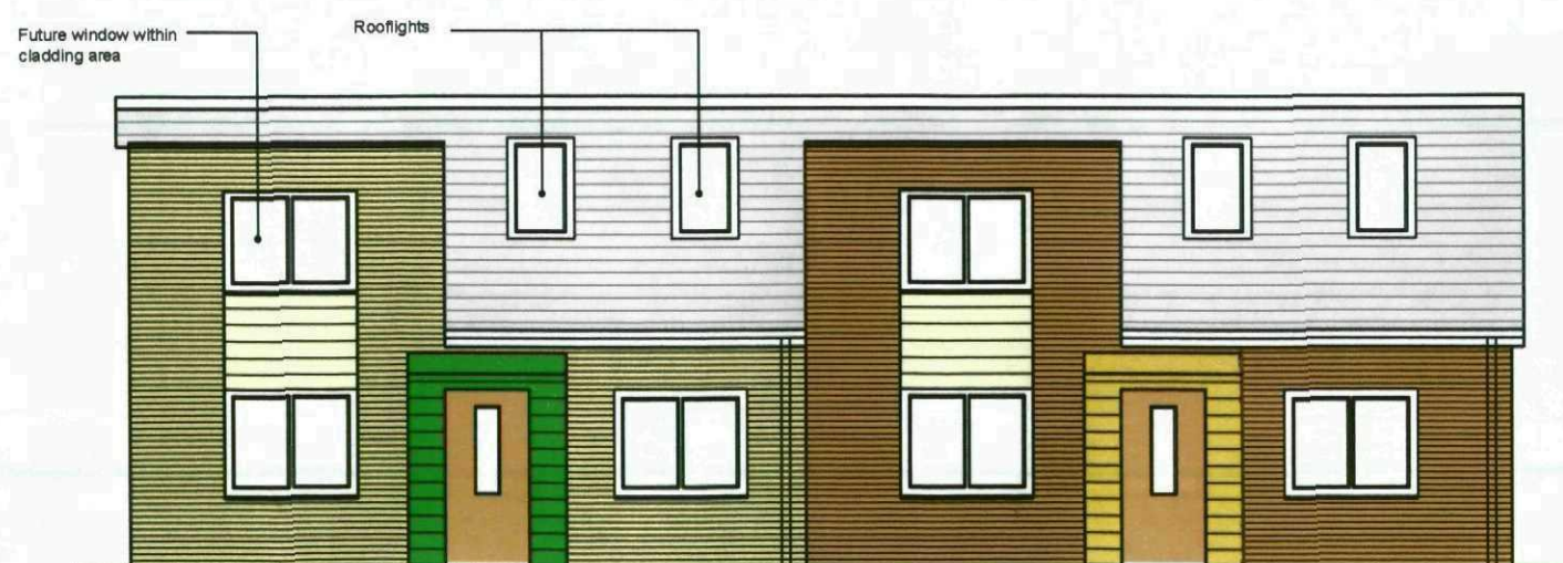
05 FRONT ELEVATION SHOWING PROPOSED ADAPTATION FROM 2B 4P BUNGALOW INTO 3B 5P BUNGALOW 04 1:100 @ A3
