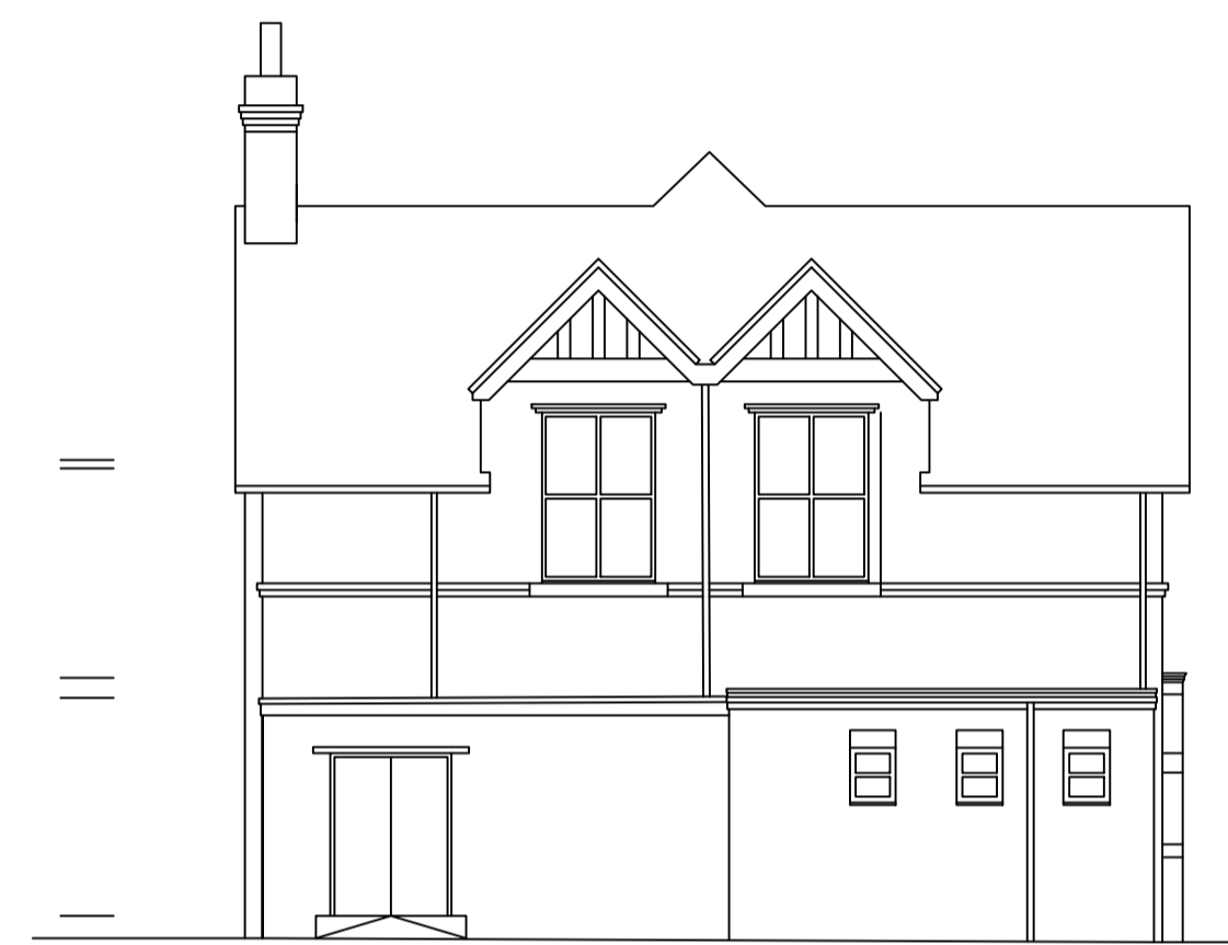
EXISTING SIDE ELEVATION
