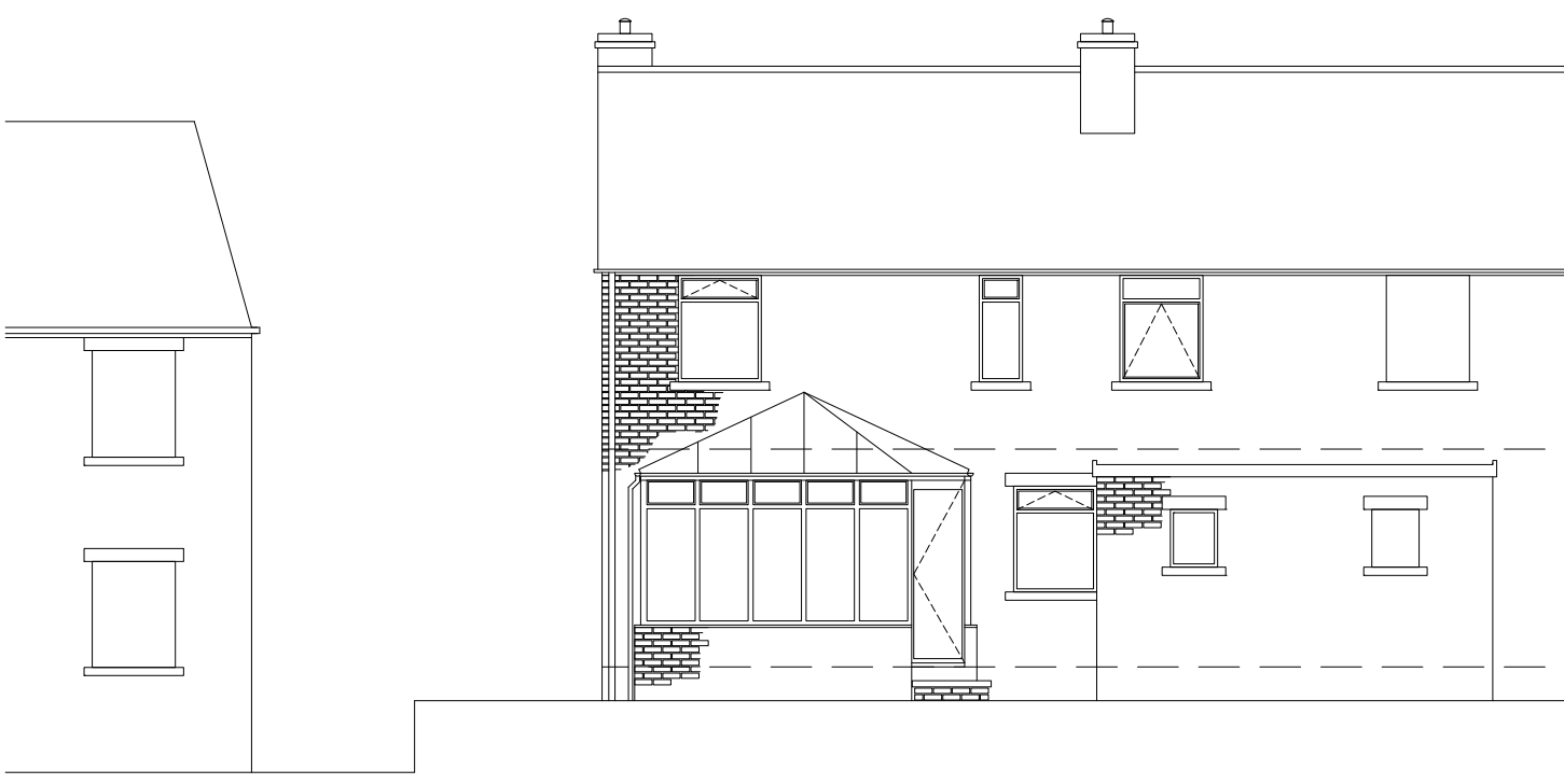
EXISTING NORTH ELEVATION
