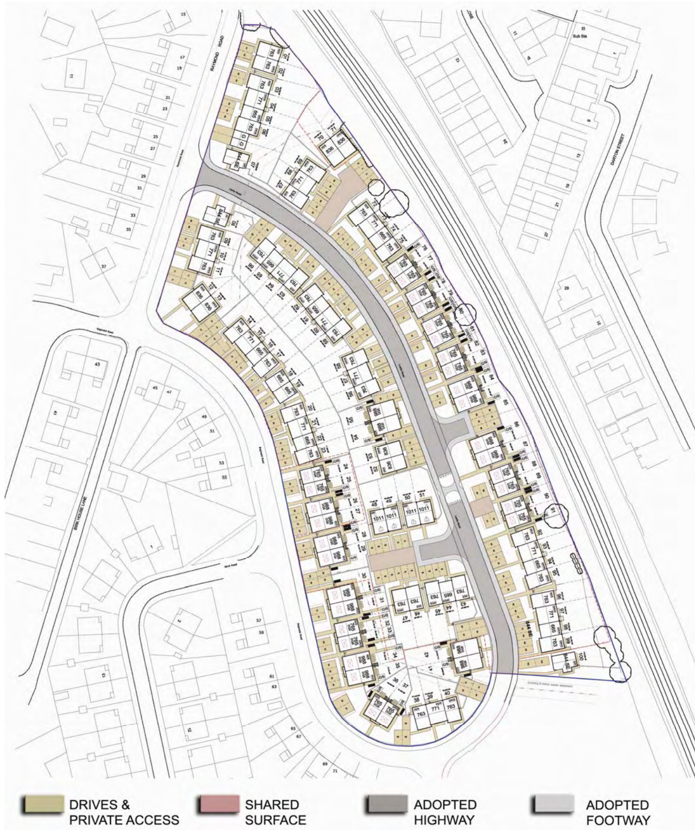
(Fig. 4.4.1) Proposed road layout showing the different surface materials excluding approved areas shown grey
