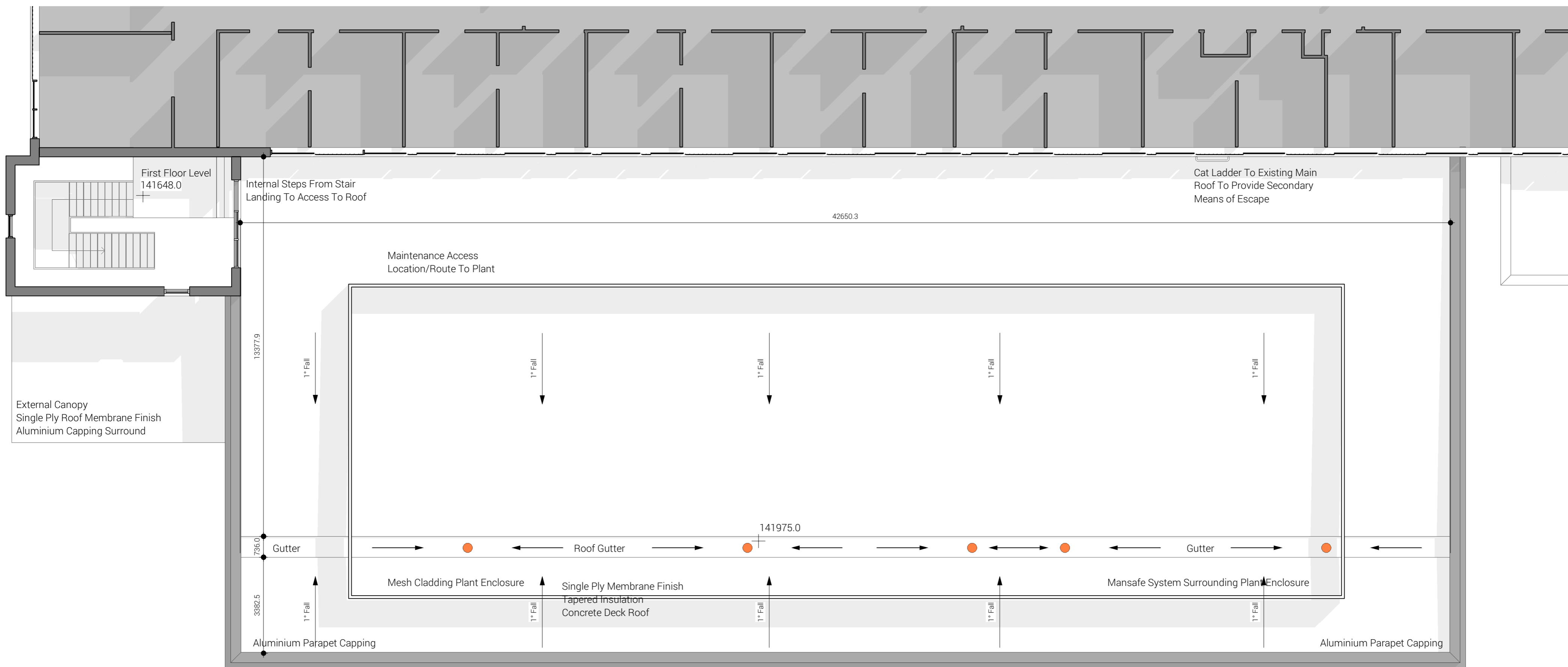
Level 1 Roof Plan 1 : 100
