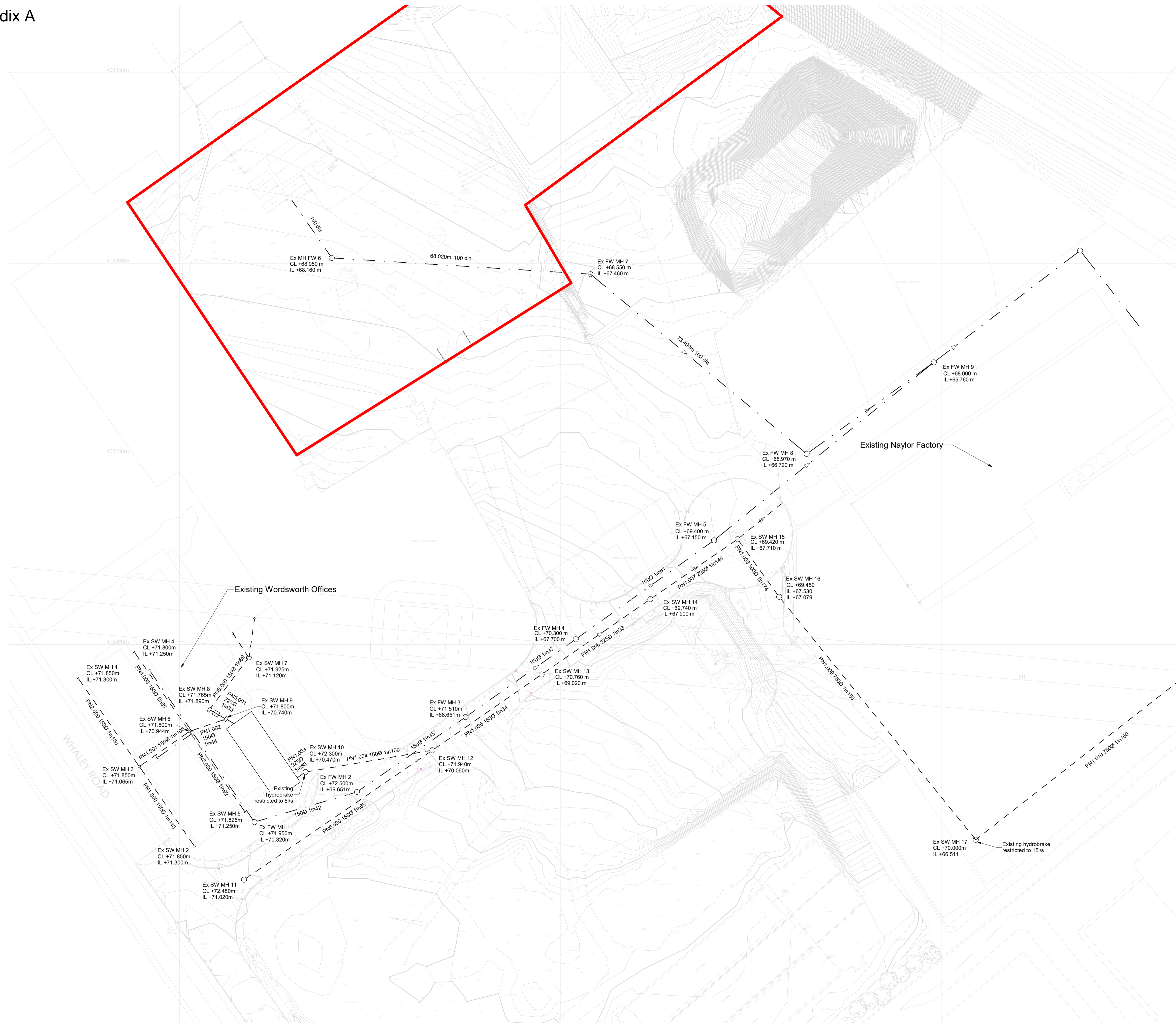
1 Existing Drainage Layout 1 : 500
