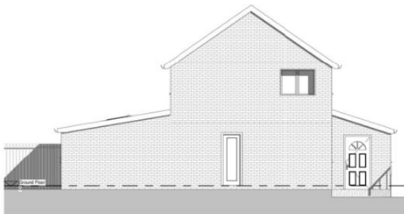
Proposed Left Elevation 1 : 50
