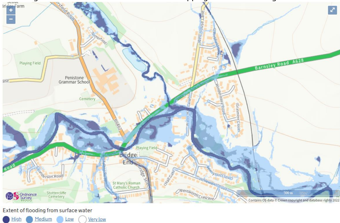
Figure 2.2 - Risk of Flooding from Surface Water Mapping
