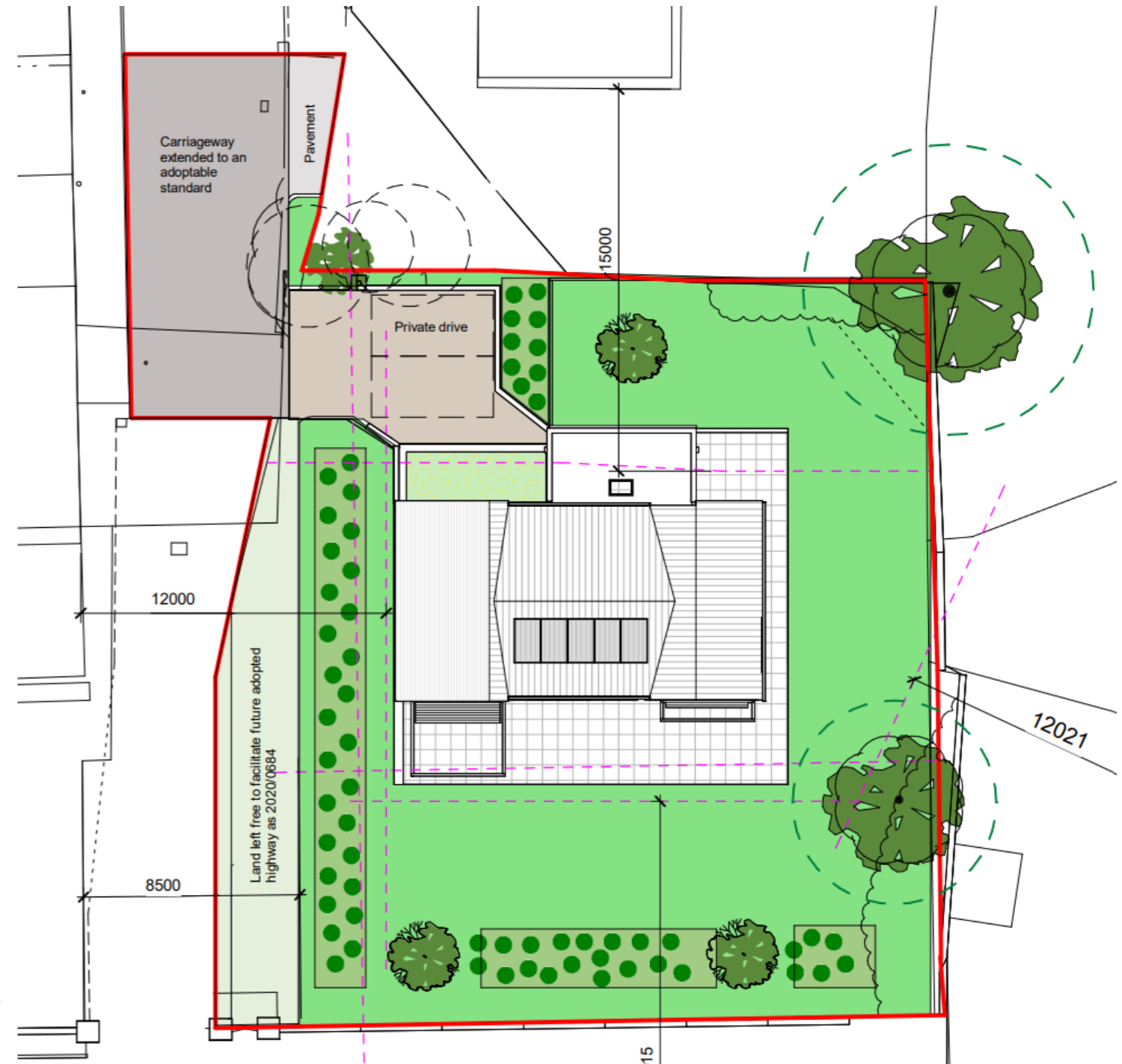
AMENDED APPLICATION PLAN - Extract from 23-122-110 rev C Tower Street Proposed Site plan
