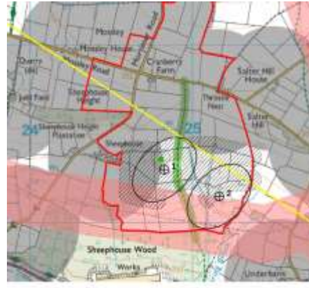
Alternative 2 – Two Repower MM82 Turbines (100m to tip; 82m diameter blades; total 4MW)
