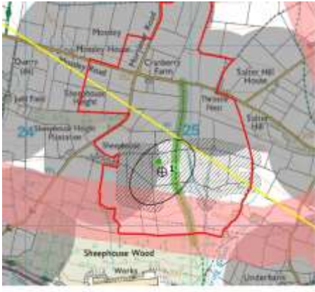
Alternative 1 – Single Repower MM82 Turbine (100m to tip; 82m diameter blades; total 2MW)
