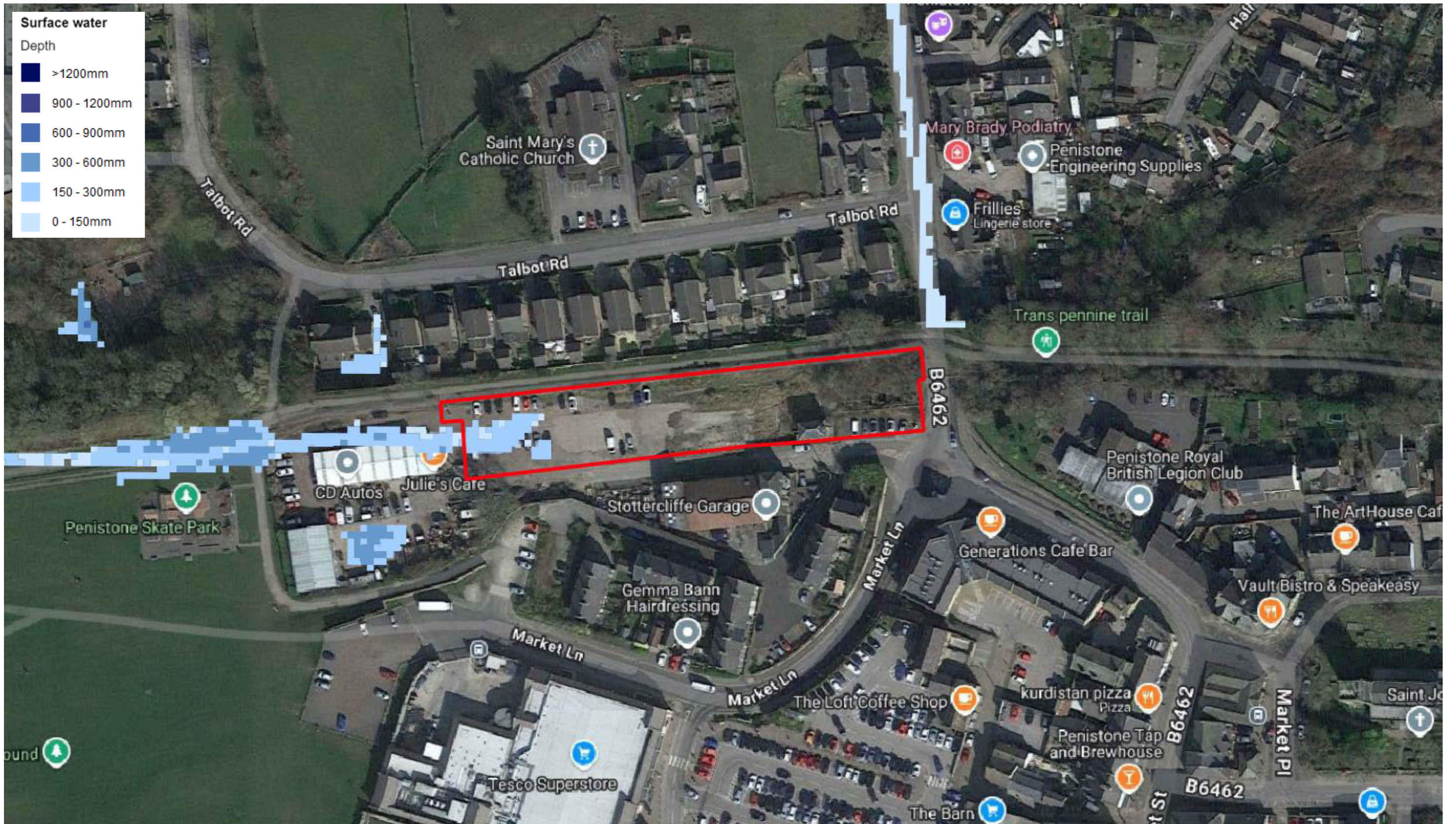
Environment Agency – Surface Water Flood Depth – High Risk Scenario (1 in 30 year event)
