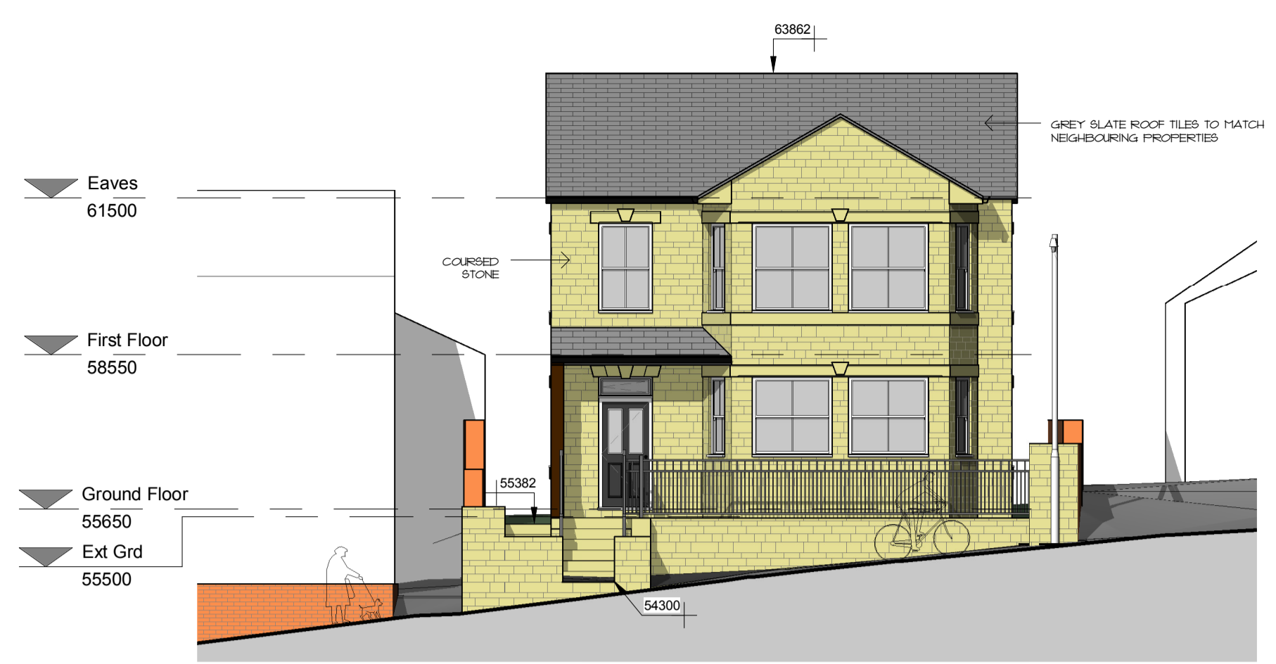
Front Elevation (NW Facing) 1 : 100
