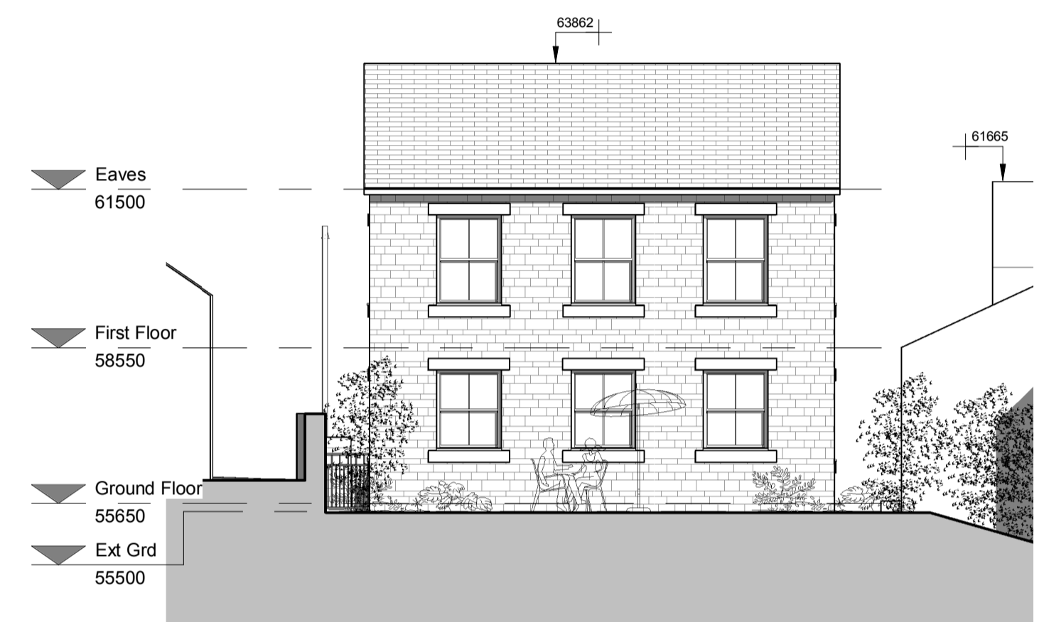
Rear Elevation (SE Facing) 1 : 100
