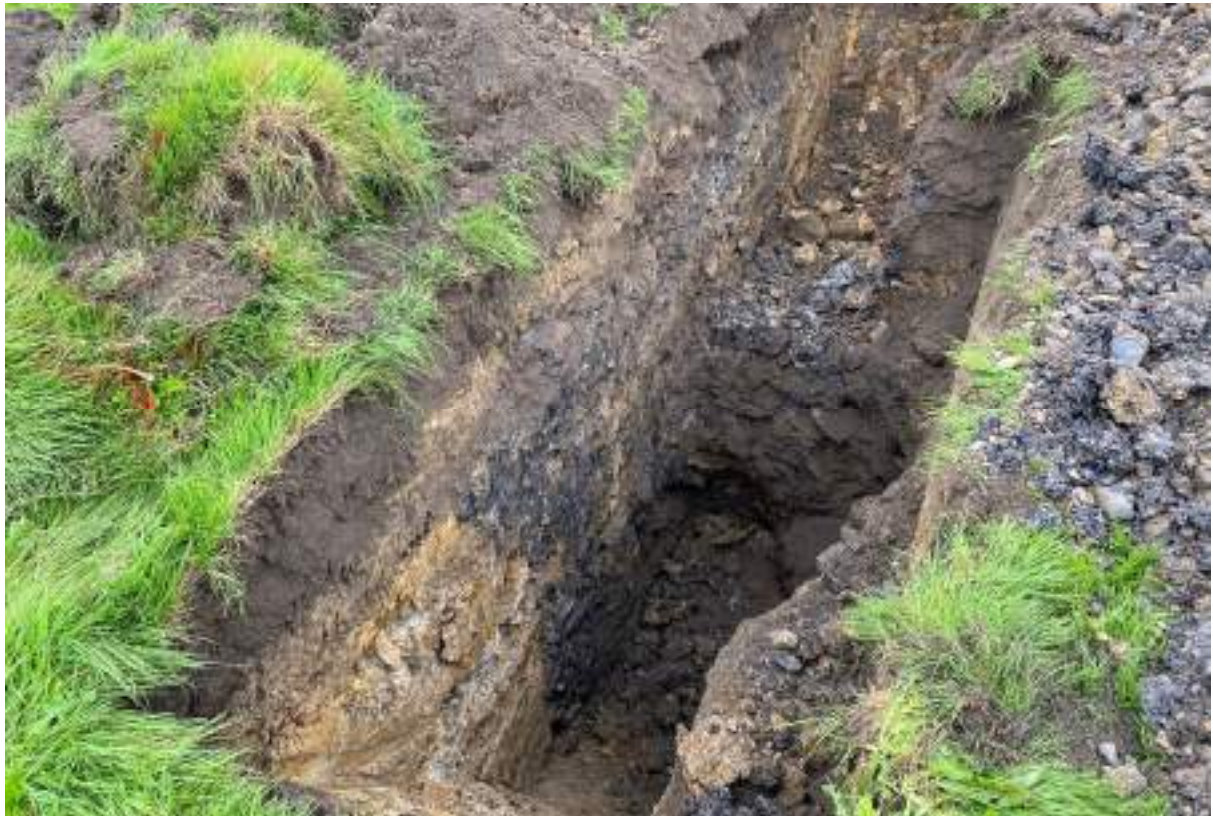
Photograph 36 – TP110 Showing change between natural and infilled shaft.
