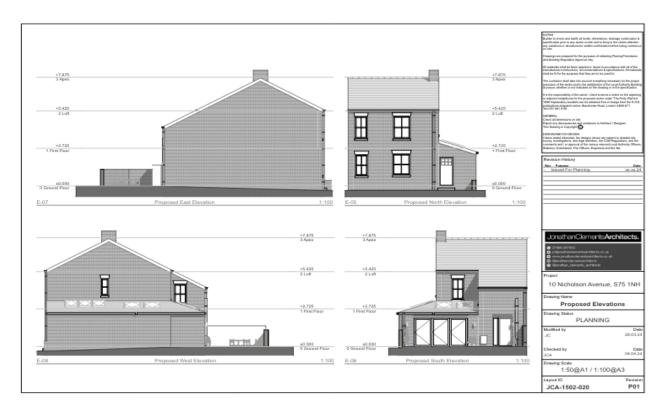
The applicant is seeking approval for the erection of a single storey wrap around side/rear extension. The extension will project 2.3 metres from the side (west) elevation and 2.15 metres from the rear elevation of the dwelling. The extension will feature a mono-pitched roof with a ridge height of 3.6 metres and an eaves height of 2.6 metres. The materials will be matching brickwork and roof tiles.
