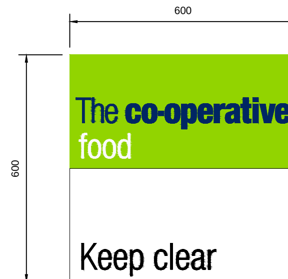
SIGN E Wall mounted Flat Panel with applied vinyl display and anti-graffitti lacquered Non illuminated SCALE 1:10
