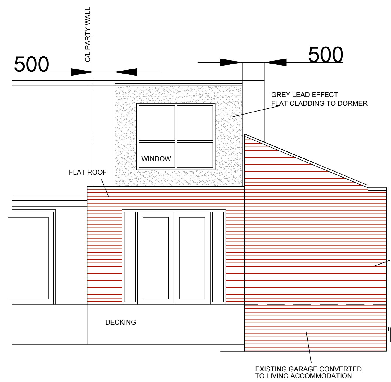
SOUTH ELEVATION - REAR
