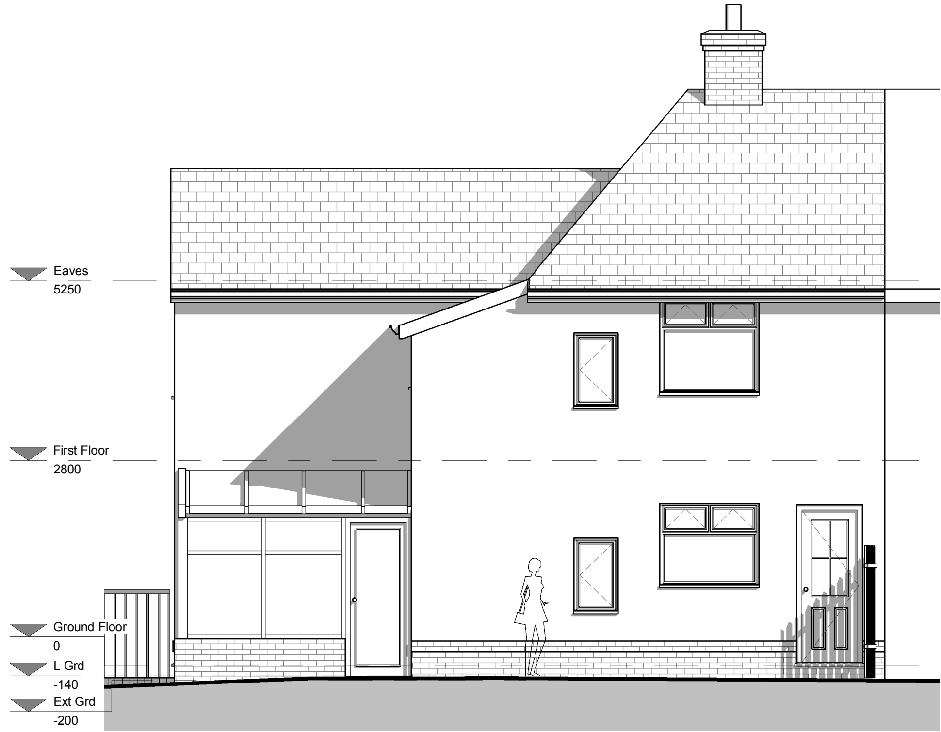
Front Elevation (South Facing) 1 : 50
