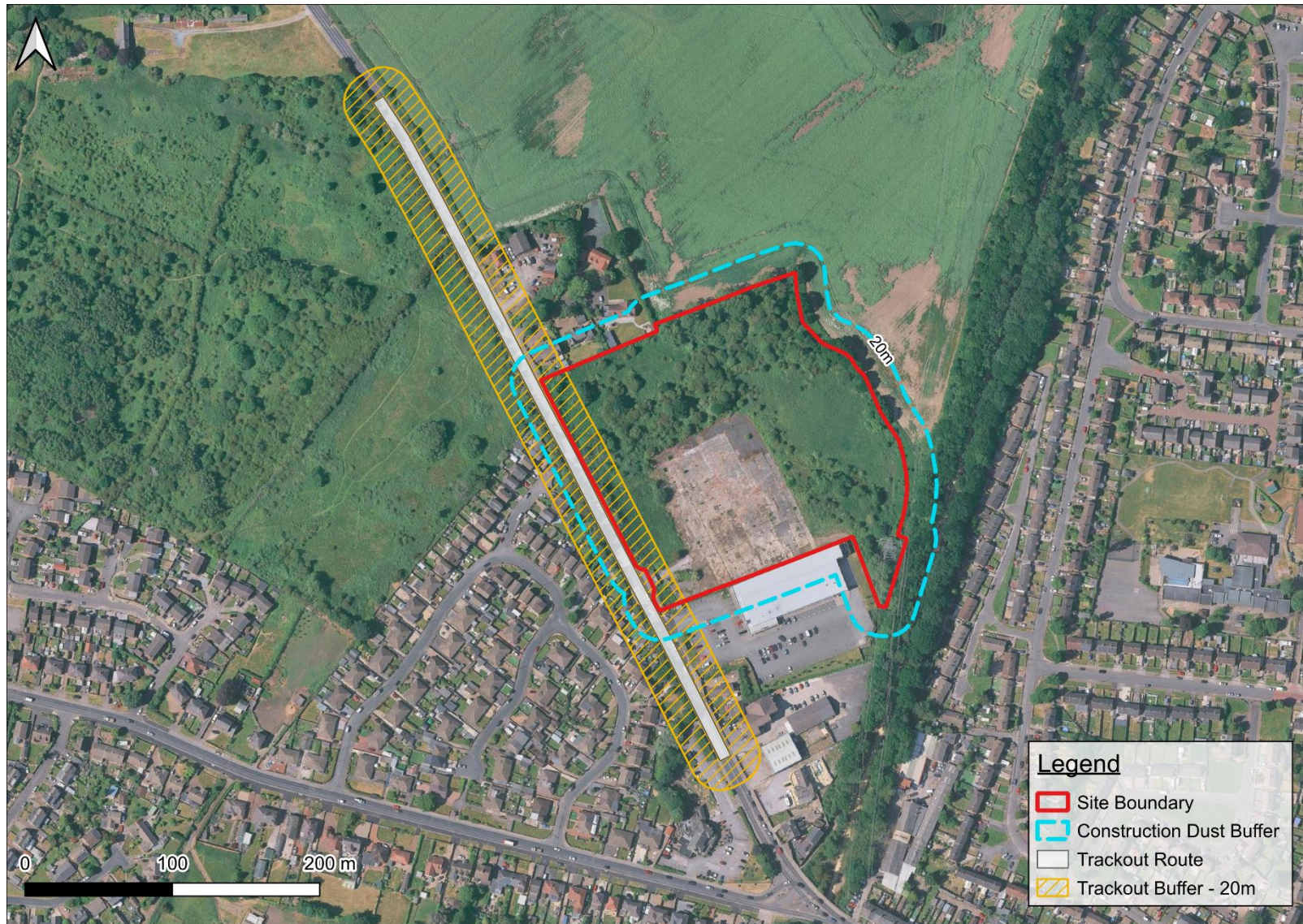
Figure 2: Construction Dust Buffers
