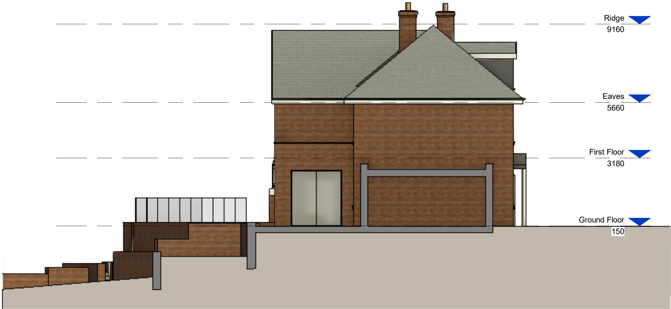
2 Proposed Side Elevation (South East) 1 : 100
