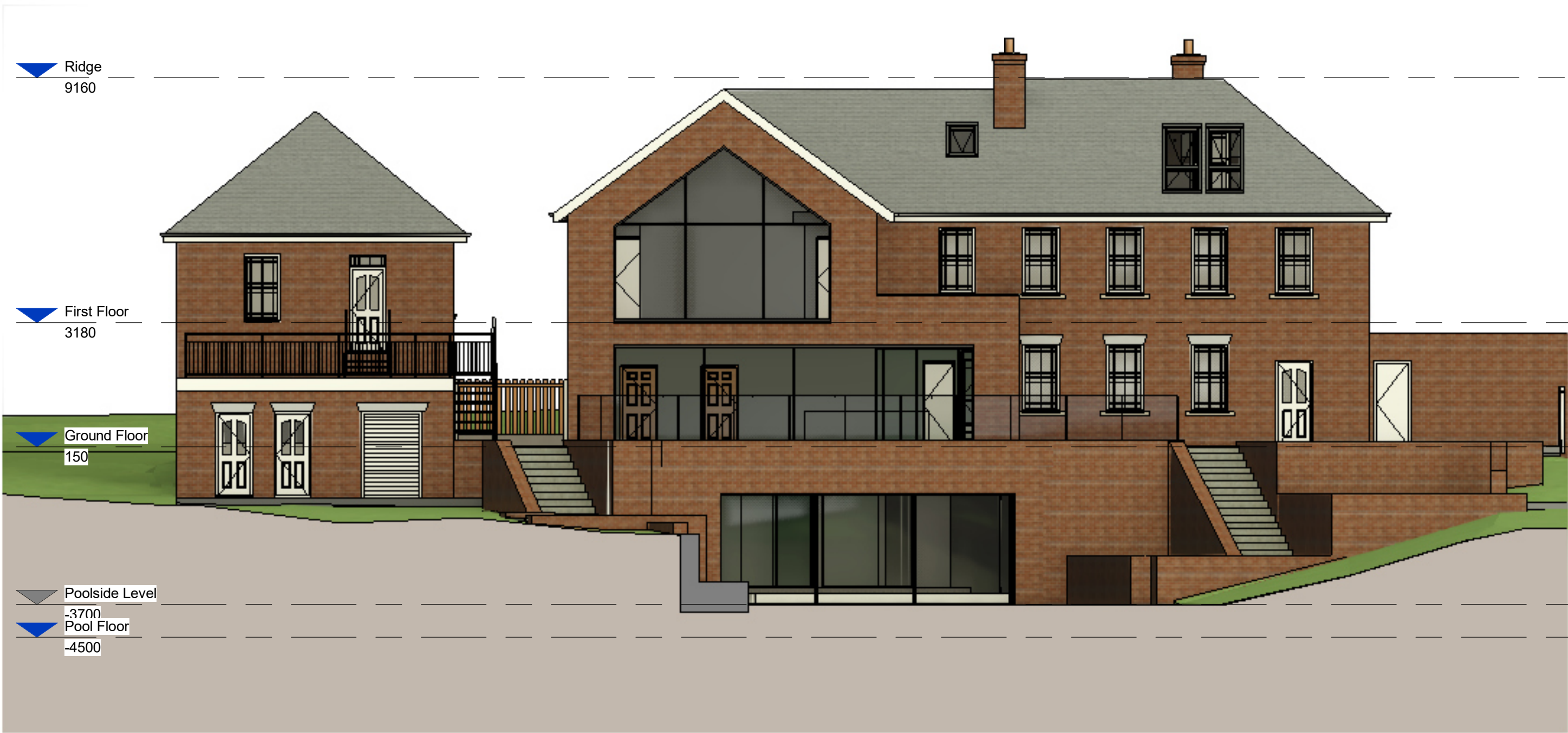
3 Proposed Rear Elevation (South West) 1 : 100
