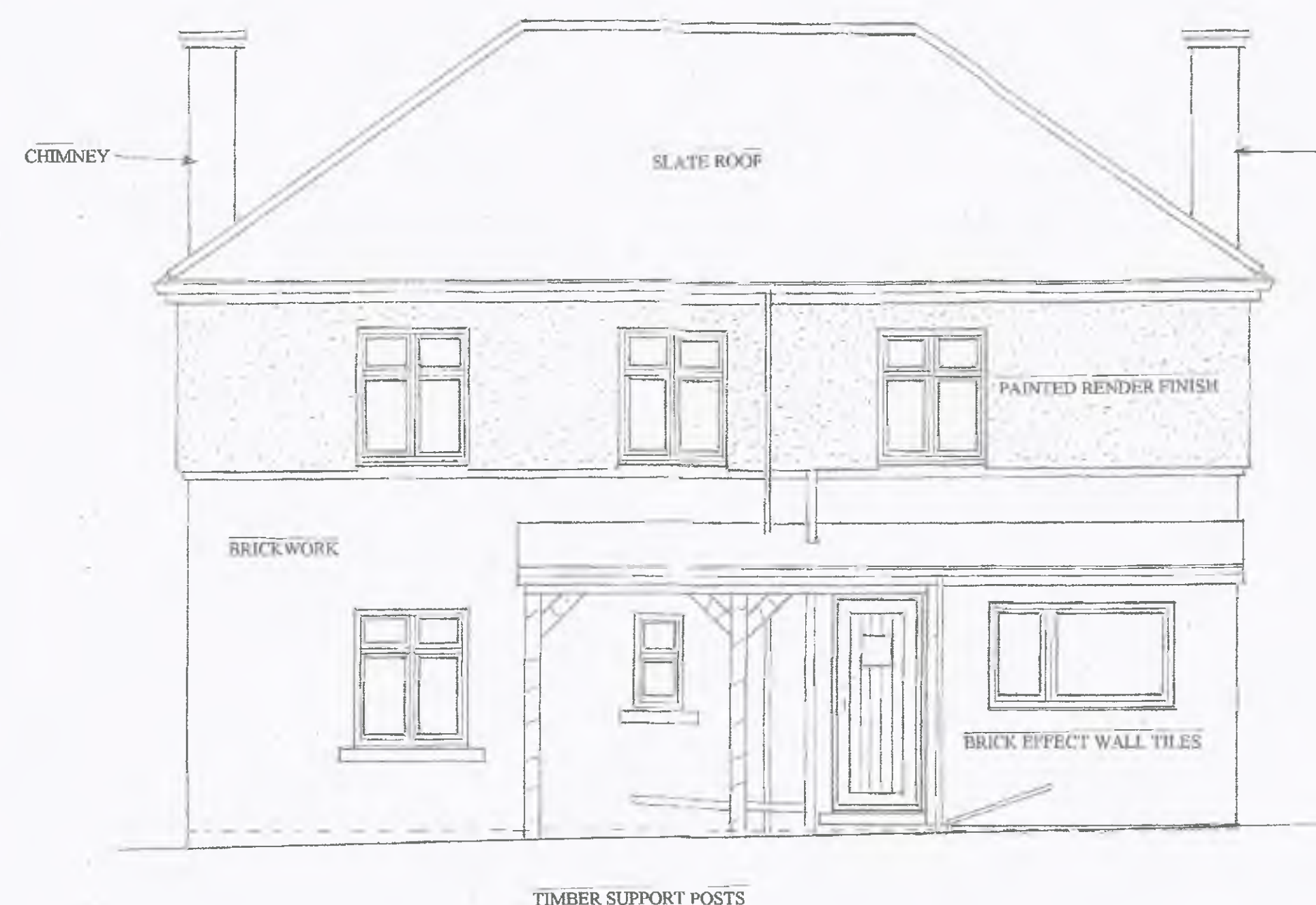
EXISTING REAR ELEVATION
