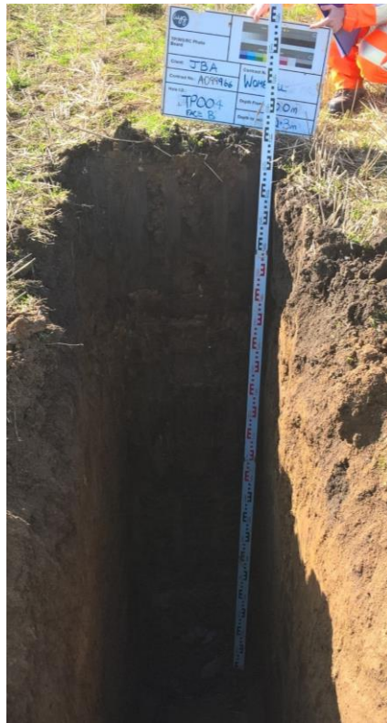
Photograph No.13: TP004 Short Face 0.0-2.3m
