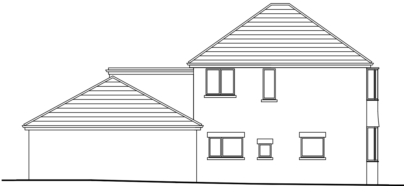
Existing Side Elevation (East Facing)
