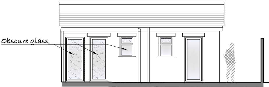
PROPOSED SOUTH ELEVATION SCALE - 1:100
