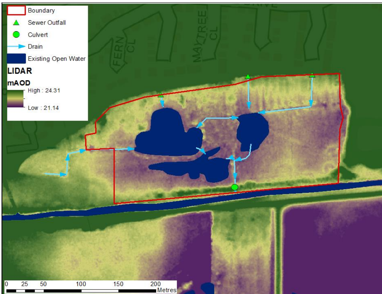
Figure 6: Existing Site Drainage
