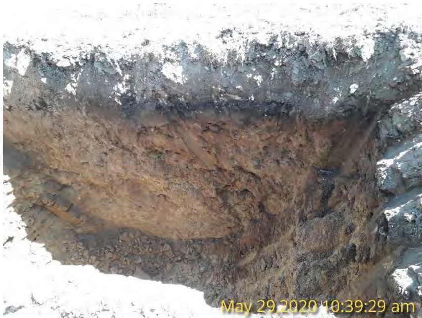
Photo 27: Ground conditions in CHP showing shallow bedrock (sandstone)
