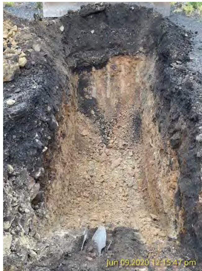
Photo 34: Coal breeze material above sandstone bedrock
