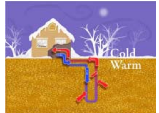
Ground Source Heat Pump
