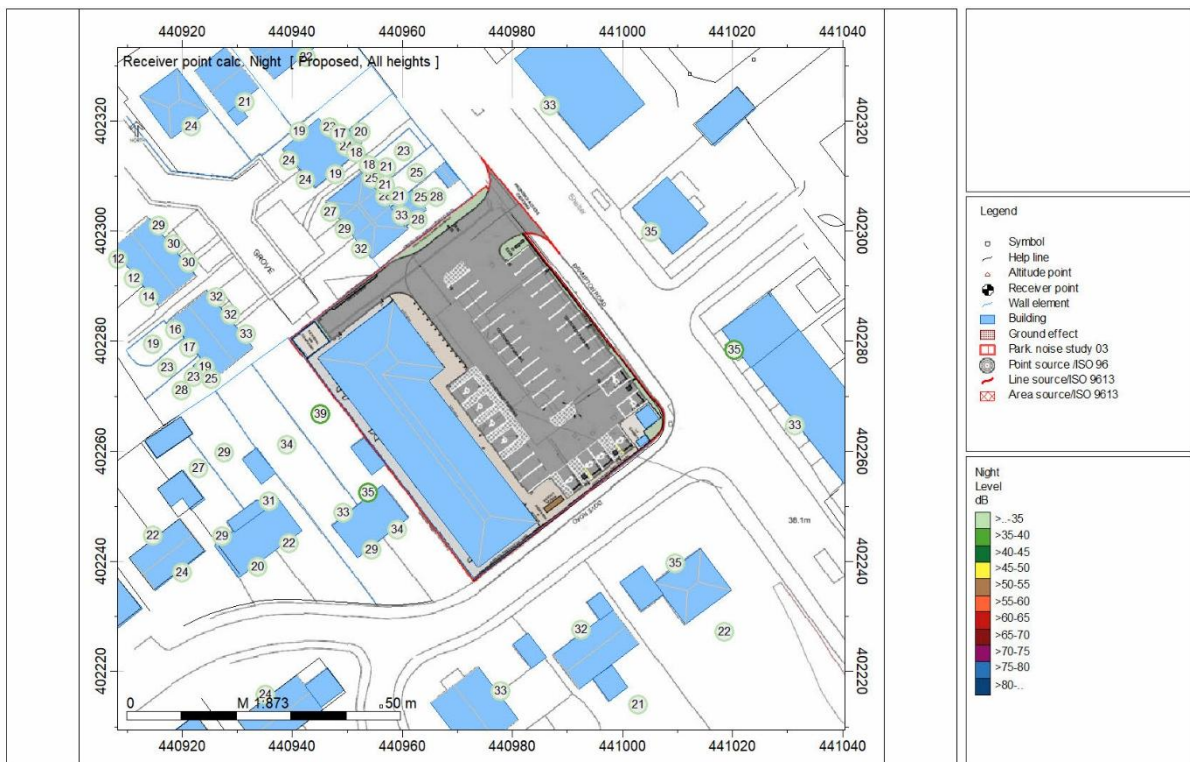
Figure E2 – IMMI Predicted Sound Pressure Levels Over Worst-Case Night-time Period (No Deliveries During Night)
