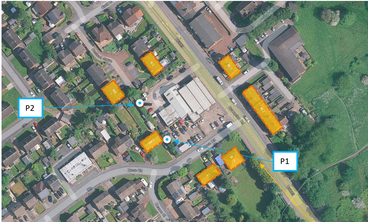
Figure B1 – Location plan with measurement positions and worst-case receptors annotated in orange
