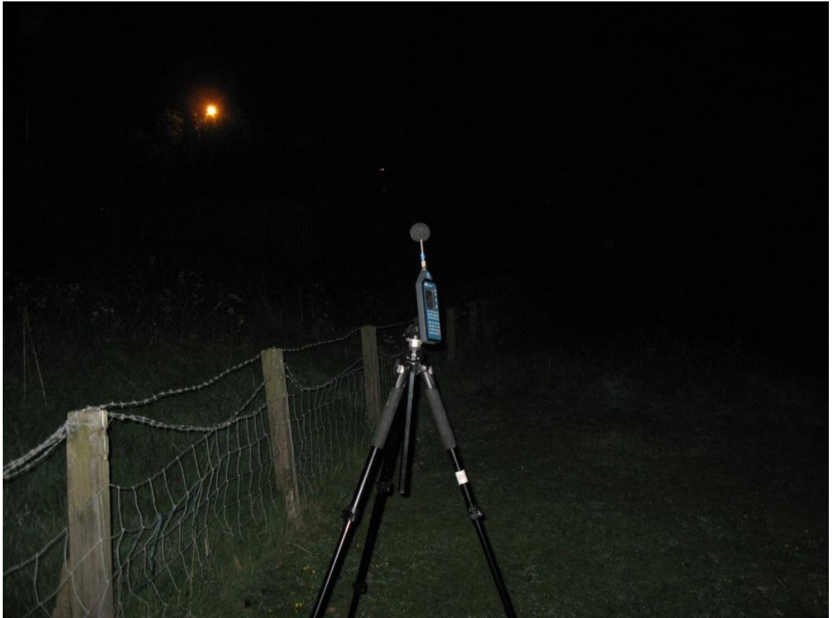
Figure 3: Background measurements in progress
