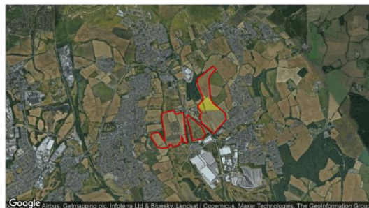
Observer Location Sun azimuth range is 272.1° - 293.1° (yellow)
