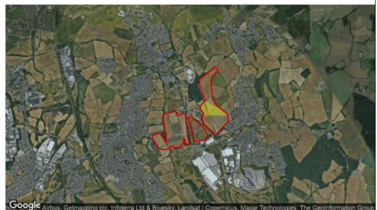
Observer Location Sun azimuth range is 272.3° - 293.8° (yellow)
