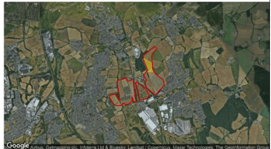
Observer Location Sun azimuth range is 270.7° - 293.5° (yellow)
