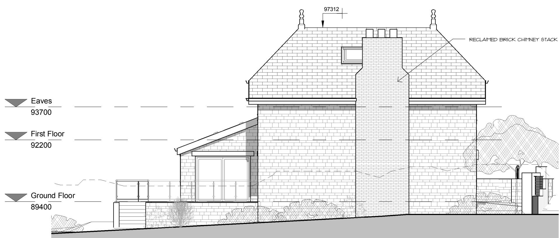
Side Elevation (SW Facing) 1 : 100
