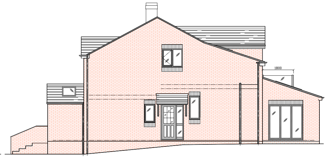
PROPOSED SIDE ELEVATION ON 'C'
