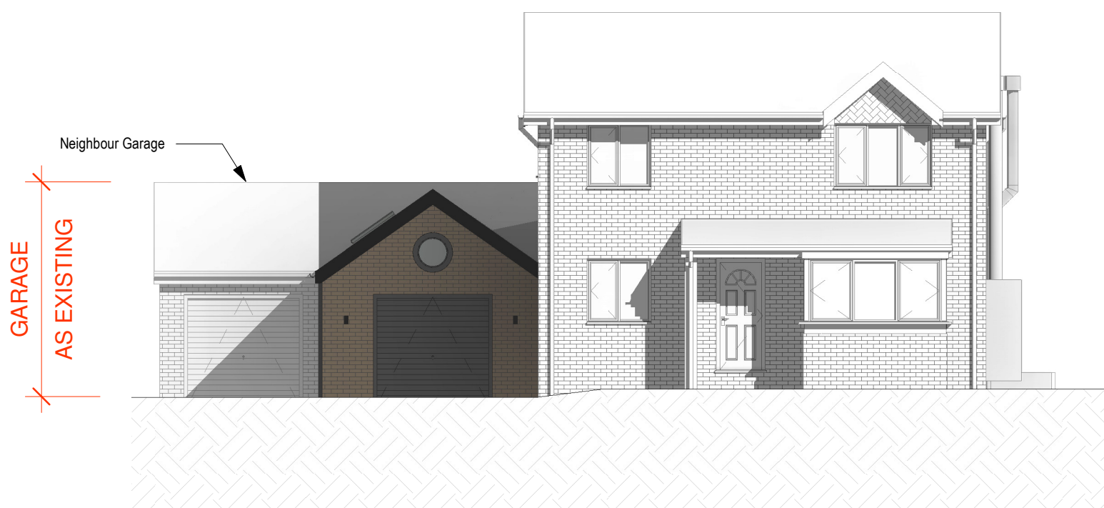
4b Proposed North West Elevation 1 : 100
