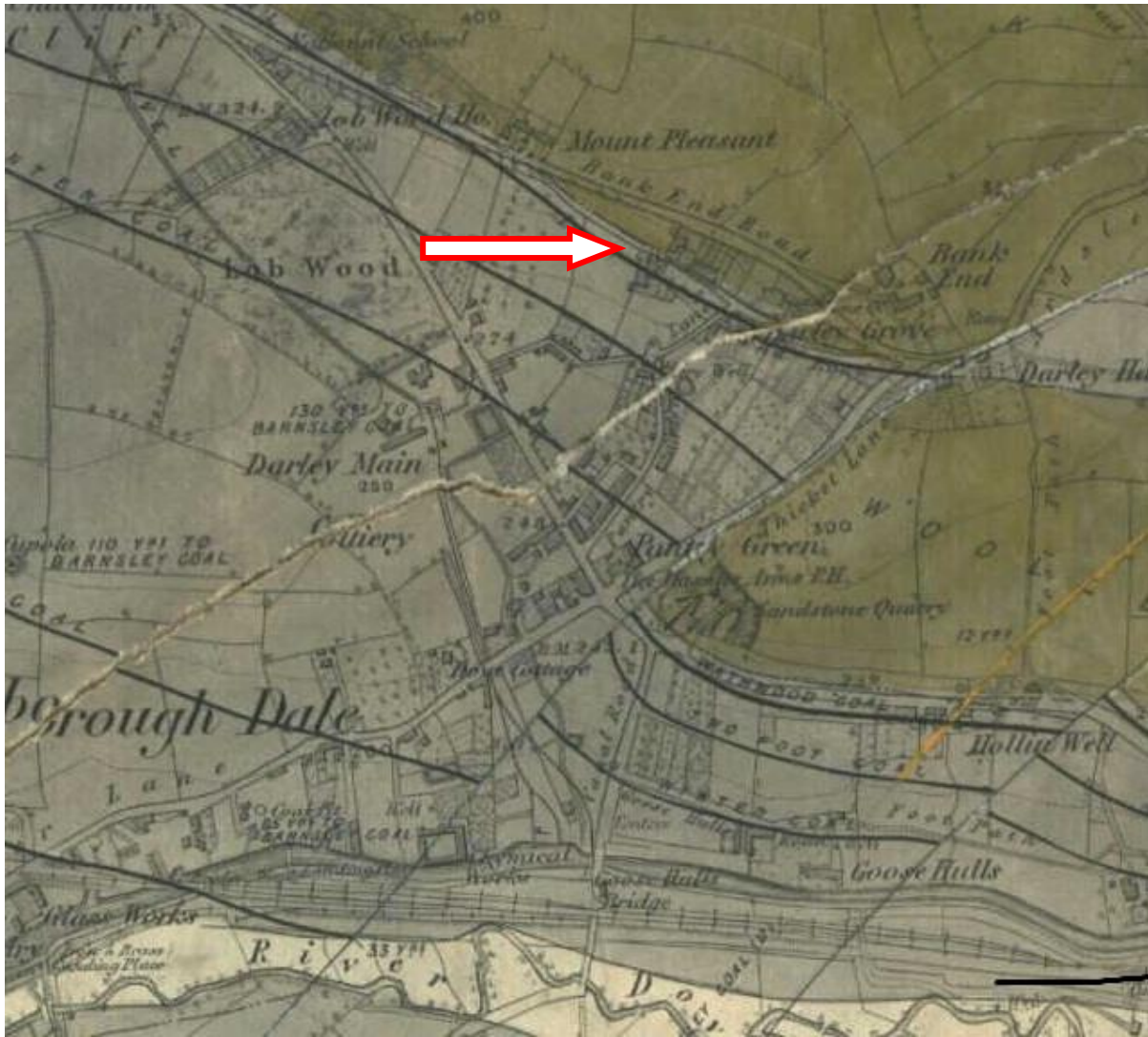
Figure 1 showing the 1 st Edition Geology Sheet 274 with the site shown by the red arrow. Note the shaft to the south west of the site is possibly Darley Main Pit. Note it is 130 yards to the Barnsley Coal and the Winter Coal is further up the hill from the Colliery so cannot have been worked from this colliery. Note the fault to the east that throws the Rock down and displaces the 3 seams south.
