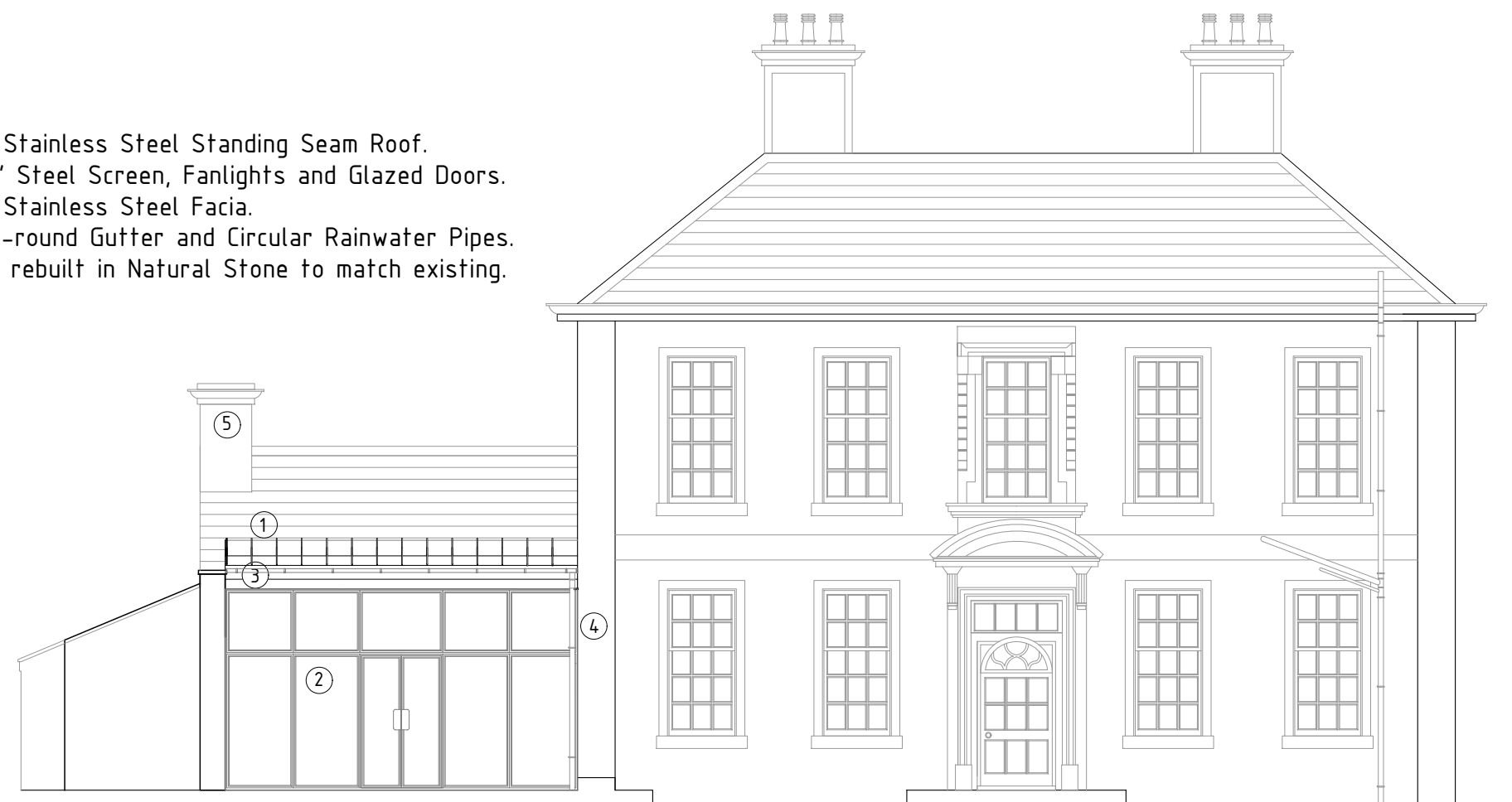
PROPOSED WEST ELEVATION
