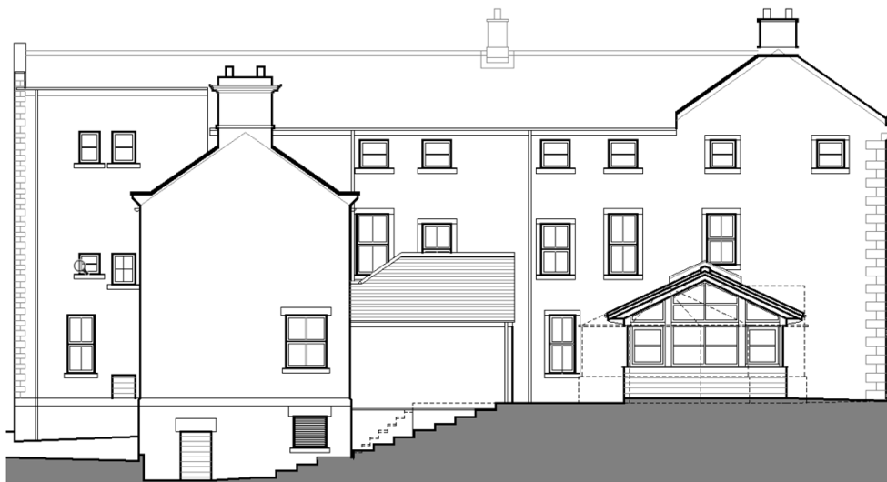
Fig 16: Proposed new conservatory roof provides balanced gable end to compliment south and north gables of existing building.
