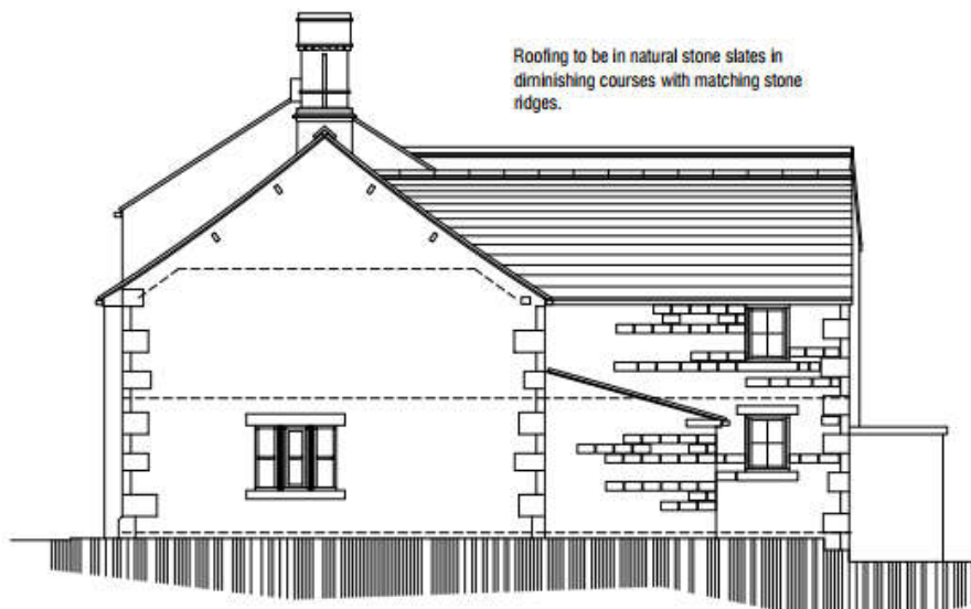
07. South Elevation showing proposed extension
