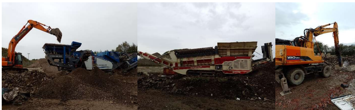
Pictures 1 – 3 (left to right) Kleeman mobile crusher/MDS M412 mobile trommel/hydraulic pecker
