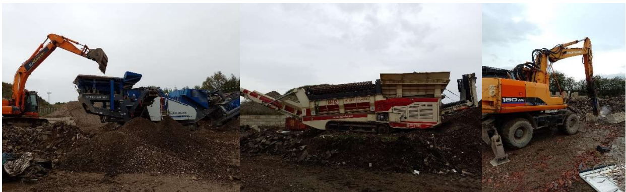
Pictures 1 – 3 (left to right) Kleeman mobile crusher/MDS M412 mobile trommel/hydraulic pecker
