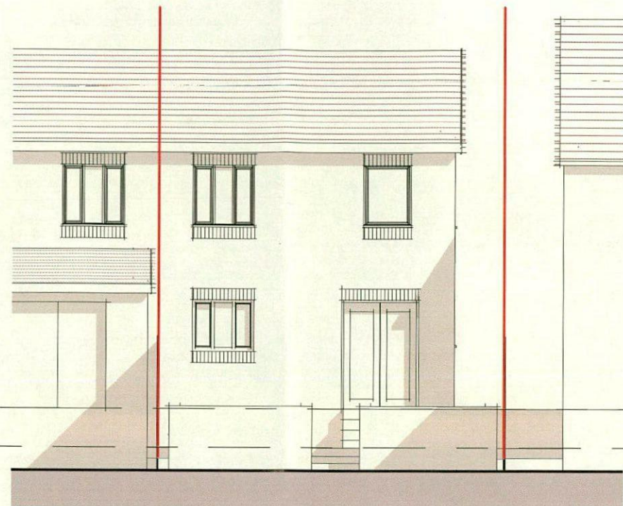
Existing Rear Elevation 1 : 100
