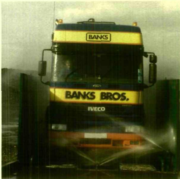
A wheel wash in action
