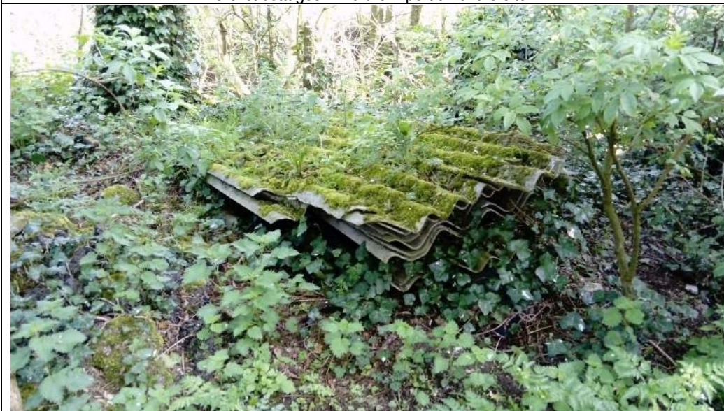
Potential asbestos containing material discarded on-site
